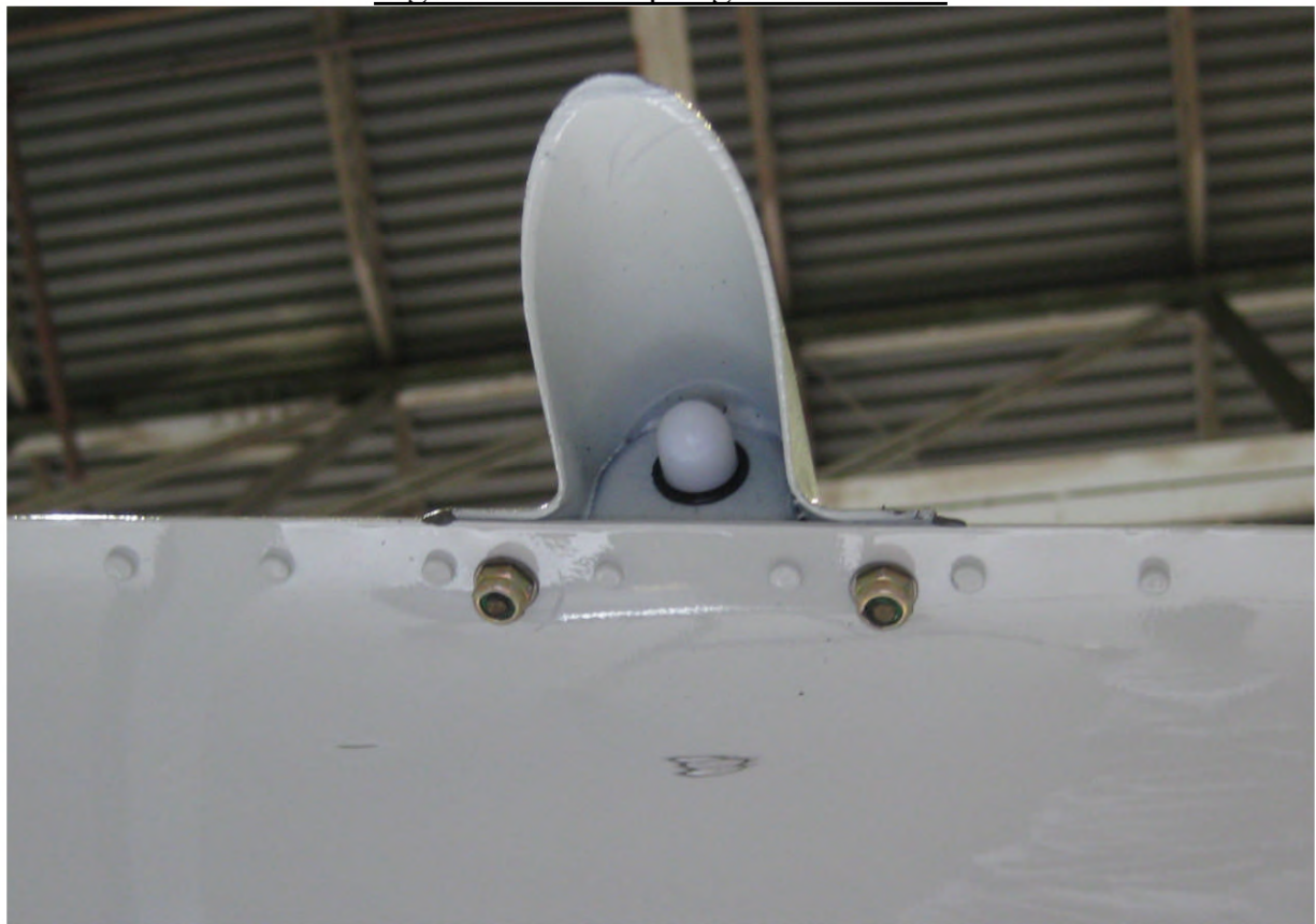
Figure 113-2: Nuts on Trailing Edge of Flap Cove
